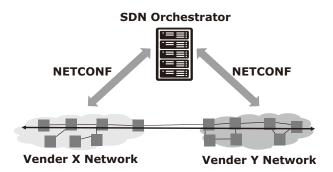
Fig. 1 Monitoring and control of devices using NETCONF.
