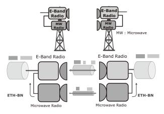
Fig. 4 Example of multiband aggregation configuration.
