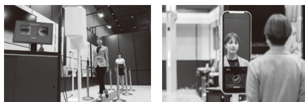
Photo 2 Demonstration of NEC's walkthrough-type iris recognition system.
