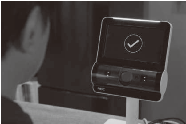
Photo 3 Multimodal biometric authentication terminals.
