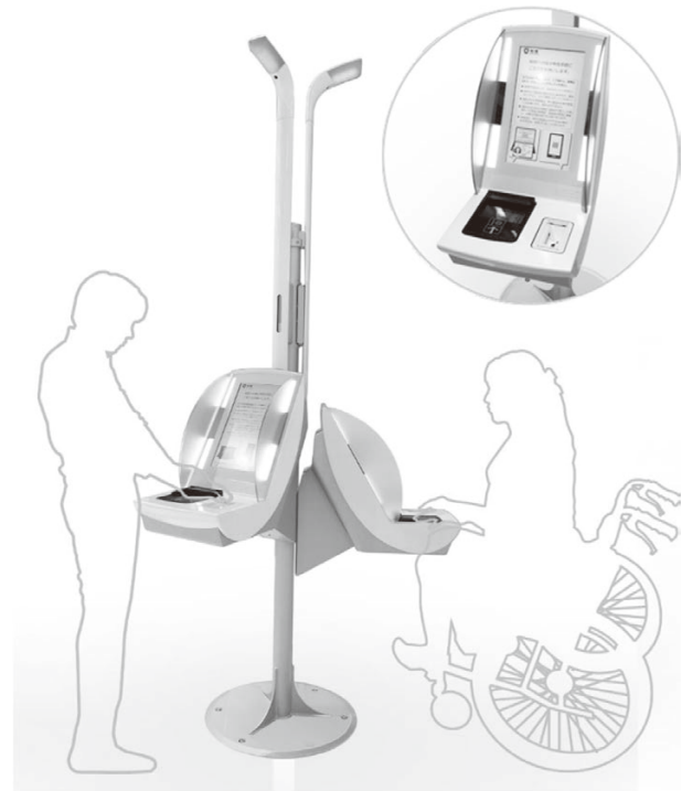
Fig. 3 Electronic Declaration Terminal with barrier-free design.
