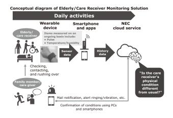
Fig.4 Conceptual diagram of Elderly/Care Receiver Monitoring Solution.
