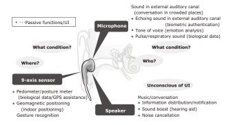
Fig. 6 Features of a hearable device.
