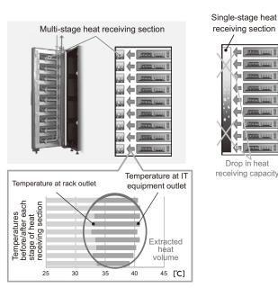
Fig. 6 Coolant circulation technology of the multi-stage heat receiving section.
