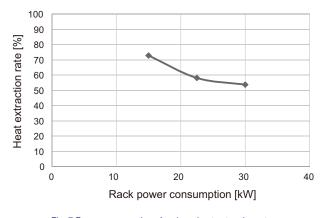
Fig. 7 Power consumption of rack vs. heat extraction rate.
