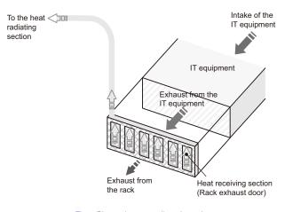
Fig. 5 Phase change cooling of a rack.
