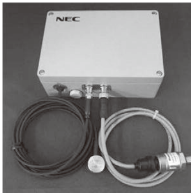
Photo Sensor unit for monitoring of water infrastructure.
