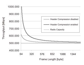
Fig. 4 Effects of header compression.
