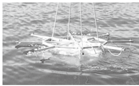
Fig. 5 Passive acoustic sensor (prototype) and main function.
