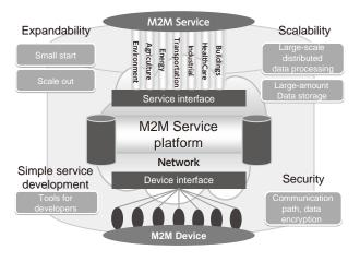
Fig. 2 CONNEXIVE M2M service platform.
