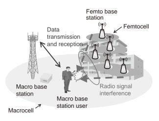
Fig. 1 Radio signal interference between femtocells and macrocells.
