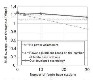
Fig. 3 Properties of the macro terminal (MUE) throughput during times of high data transmission volume at each femto base station.
