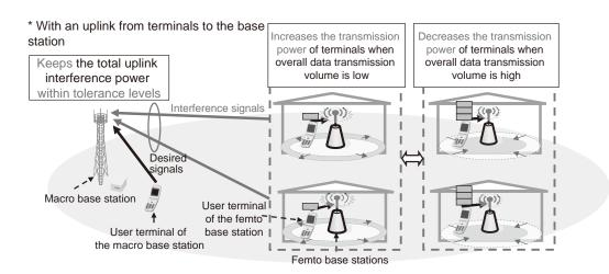
Fig. 2 Transmission power control in response to the overall data transmission volume of all femto base stations.
