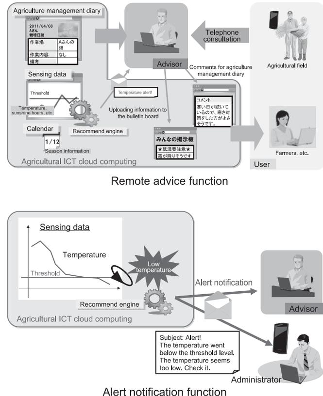
Fig. 3 Cultivation work support service using field sensing.
