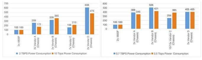
CGNAT Relative Power Consumption (in %) w.r.t FG-4800F SecGW Relative Power Consumption(in %) w.r.t. FG-4800F
