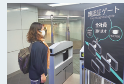
A face recognition access control system that can be used even with masked people (employee gate of NEC Head Office building)
