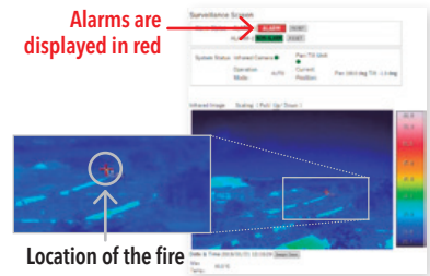
Fire detection screen image using infrared camera
