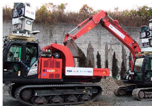
Remote control of construction machinery using 5G
